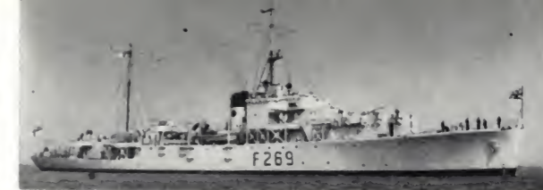
The last 'River' class to be actively employed in the Royal Navy was HMS Meon. Notice the revised gun armament, exclusively of close-range weapons, and particularly the special Oerlikon sponson above the post-war pendant number. As an HQ ship for landing craft, she had an extensive radio system, and wore the 'Combined Ops' badge on her funnel beneath the 'leaders' band.
